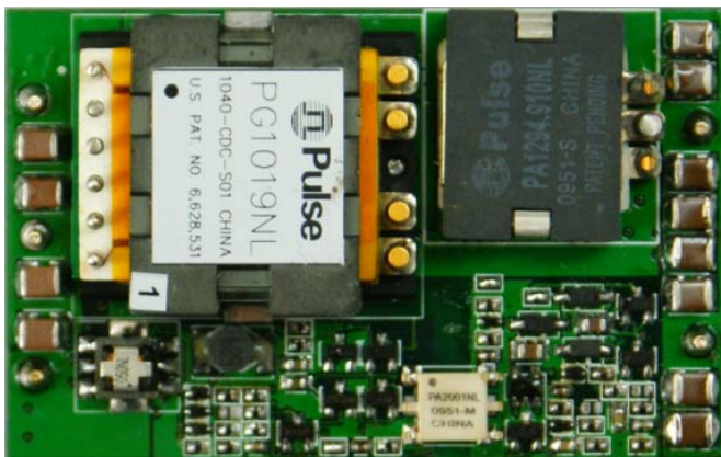
FIGURE 1. TOP VIEW OF ISL6726EVAL1Z (ACTUAL SIZE: 40x60x16mm)
